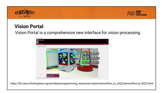
For FTC Blocks and Java teams, VisionPortal offers key capabilities of AprilTag and EasyOpenCV, along with TensorFlow Object Detection (TFOD) – at the same time!
