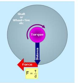
**Torque** (T) roughly quantifies the turning force on an object like a gear or a wheel. Torque is commonly expressed in units of [Nm],  $[oz \cdot in]$ , or  $[in \cdot lbs]$ .
